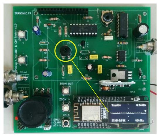
**Trick**: You can force the trigger by moving the line up with the **Position** potentiometer RV2.
