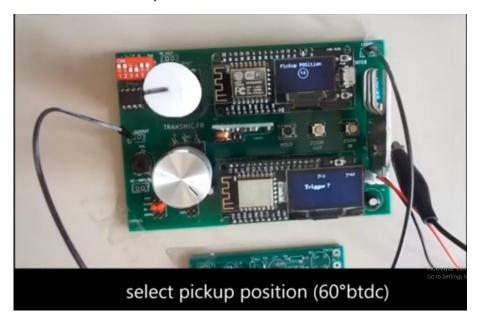
Set the pickup position at 60 degree btdc by turning the top potentiometer and pressing the top right button (enter) of the CDI Simulator/Analyser (top display)
