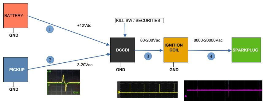
Use a SCOPE or a DVA multimeter to measure voltage at points 2,3
