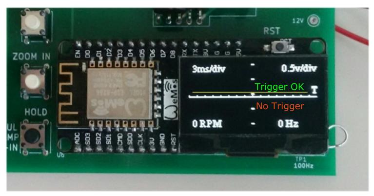
**Trigger level** decide when acquisition and display begin. When the input signal is higher than trigger level, signal is captured and display is steady.
